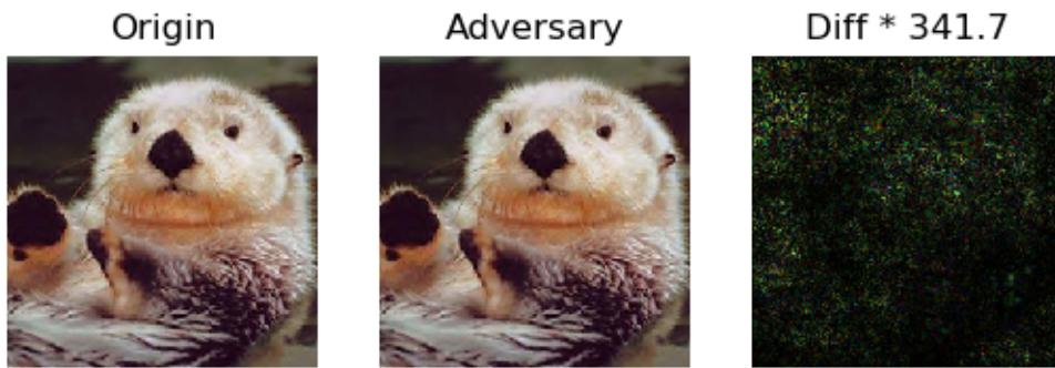
Above example shows that it is easy to fool a well-tuned classifier by adding small perturbation to the target.
